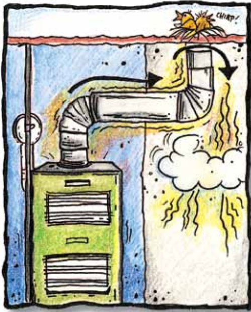
Blocked furnace vent
